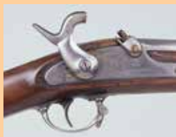
Position the hammer in full-cock position.
