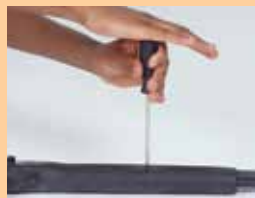
Remove the barrel key from the forearm.
